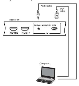
3 Connect one end of an audio cable with a stereo mini-plug (not included) to the PC/DVI AUDIO IN jack on the back of the TV, then connect the other end of the cable to the AUDIO OUT jack on the computer.
